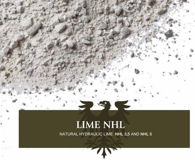
CALCE NHL 3,5 is a natural hydraulic lime NHL3,5 it complies with the current regulations UNI EN 459-1/2010 it is obtained by heating layers of calcareous marl in traditional furnaces at 1100°C. Calce NHL3,5, has in its chemical composition silica dicalcium and calcium Hydroxide typical of the natural hydraulic limes while compounds of clinker and soluble salts are absent.
